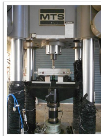
Figure 2 Three point bending test on notched prism specimen
